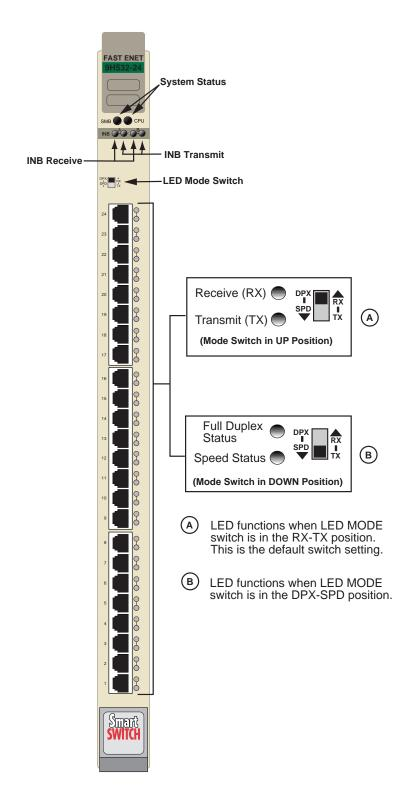
Figure 4-1. The LANVIEW LEDs (9H532-24 shown) and LED Mode Switch
